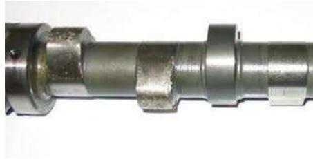
Wear: irreversible loss of material from contacting surfaces
