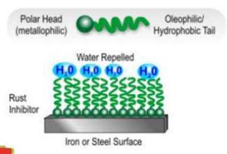
**Corrosion Inhibitors** protect copper, tin and lead-based bearing metals by neutralizing acids and by sealing surfaces from contact with water and corrosive acids.
