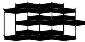
Hexagonal lattice structure of graphite
