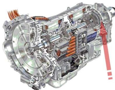
Automatic transmission of a hybrid vehicle
